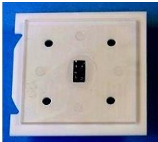
Figure 1 Top view of FLDSC chip. The large square is the ceramic, the slightly smaller square is the plastic cover.
