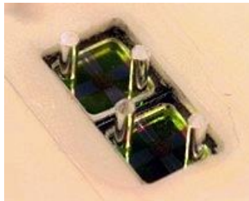
Figure 2 Close-up of the cavities and cover, showing the inlet and outlet holes for the liquid.
