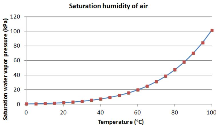
Figure 2: Saturation partial pressure of water vapor vs temperature.
