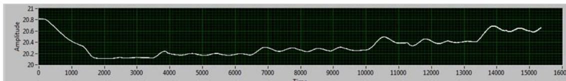
**Figure 3:** Transfer of the XEN-3880 for measurements at ever increasing absolute humidity in kPa. Transients in humidity do not show in the transfer of the XEN-5320 around 20 kPa partial water vapor pressure (measurement 2000-3000), but do show when the humidity levels are higher (later measurements), as indicated in Fig. 1. Also the absolute value of the transfer increases at higher measurement (= water vapor partial pressures) numbers, as indicated in Fig. 1.
